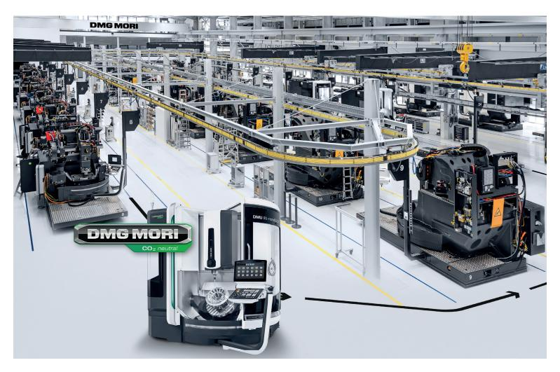
**Most modern assembly line worldwide:** The new monoBLOCK Excellence Factory went into operation at the beginning of September. Digitally and fully automated, it can now produce up to 1,000 machine tools per year. The core of the 4,000 m², highly modern flowline assembly in Pfronten is an automated guided vehicle (AGV) transport system. From 2021, DMG MORI will produce all machines worldwide completely climate-neutrally.
