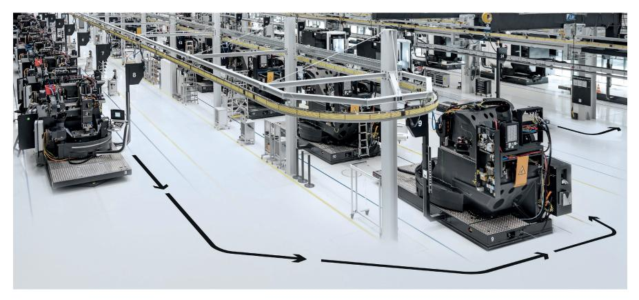
**Digital and automated:** The flow assembly with 34 AGVs in the new monoBLOCK Excellence Factory at DECKEL MAHO Pfronten increases productivity by 30%.
