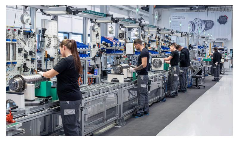
**Cycle-timed spindle assembly:** DMG MORI employees assemble more than 4,000 speedMaster spindles per year on modern high-tech workstations. As the centerpiece of every machine tool, motor spindles have an enormous impact on the precision and surface quality of the workpieces.
