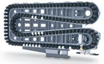
The new toolstar magazine from DMG MORI provides quick tool changing times and high-wear resistance combined with a compact design. With only 0.9 secs tool changing time, it has enough space for 30, 60 or 120 tools. The roller bearing, anti-wear chain with servo drive enables chain speeds of up to 400 tools per minute.
