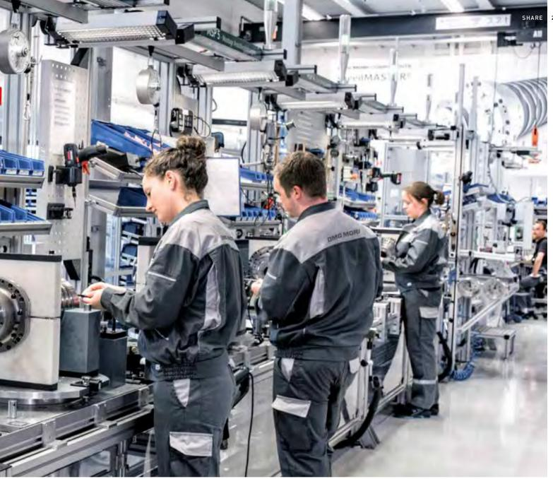
**Cycle-timed spindle assembly:** DMG MORI employees assemble more than 4,000 speedMaster spindles per year on modern high-tech workstations. As the centerpiece of every machine tool, motor spindles have an enormous impact on the precision and surface quality of the workpieces. Their sturdiness and long-term precision directly impacts the reliability and utilization ratio of machine tools.
