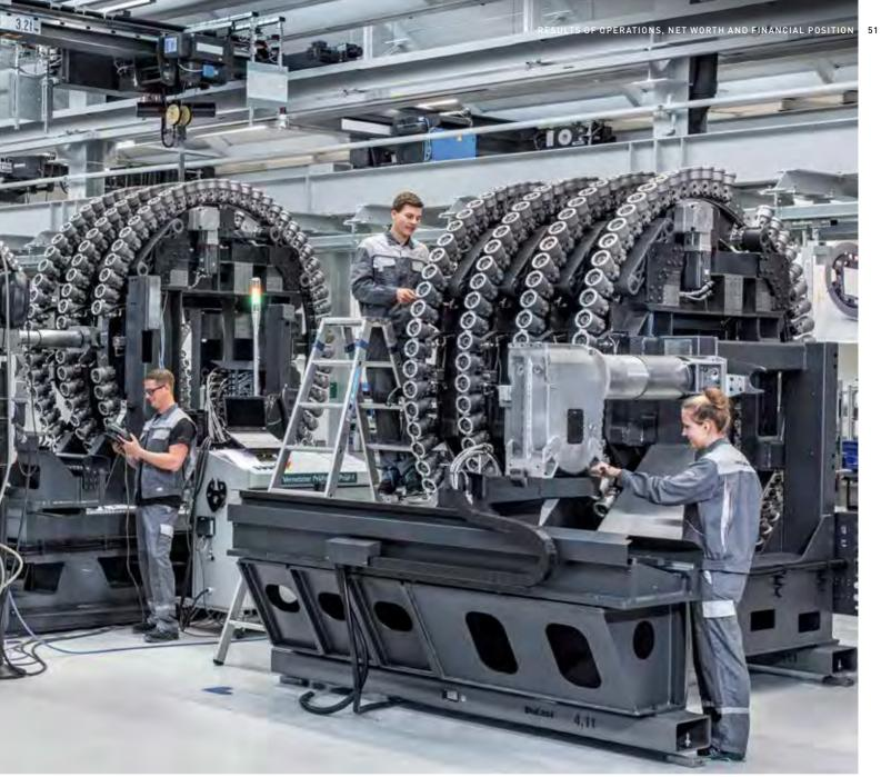
High-precision work at DMG MORI: Employees at DECKEL MAHO in Pfronten adjust the modular, patented wheel magazine with space for over 450 tools for the duoBLOCK series. In the pre-assembly, DMG MORI already lays the foundation to ensure that our core components are absolutely precise and extremely robust.
