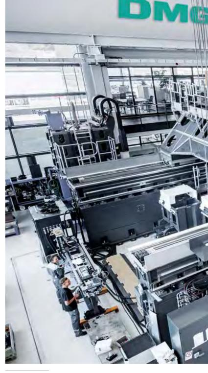
Machines for processing large-size workpieces: In the XXL machine assembly hall, DMG MORI produces, among others, the DMU 600 Gantry. The 5-axis universal processing center is comparable to a two-story detached house in size and is the largest machine in DMG MORI's portfolio. The machine provides highest precision despite a maximum table load of 150 tons. The machine uses a linear motor for quick and accurate positioning and achieves a precision of 25  $\mu m$ .
