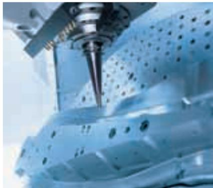
**CNC universal milling machines for 5-axis machining.**
