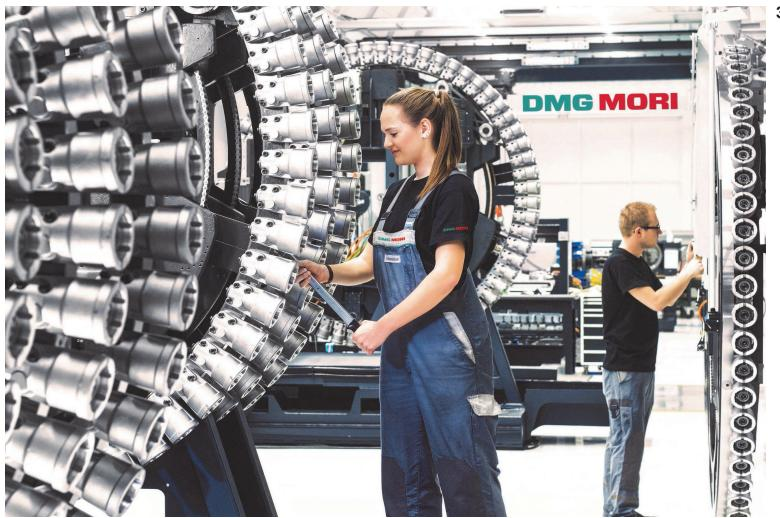
**High-precision work at DMG MORI:** Franziska Dreier, industrial mechanic at DECKEL MAHO in Pfronten, adjusts the modular patented wheel tool magazine for the duoBLOCK series with space for over 450 tools.
