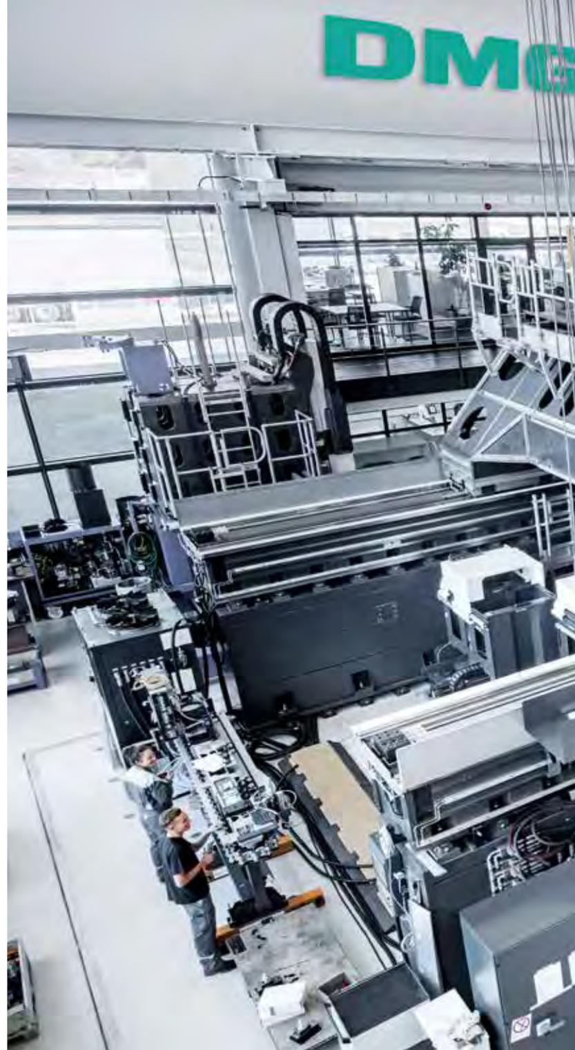
**Machines for processing large-size workpieces:** In the XXL machine assembly hall, DMG MORI produces, among others, the DMU 600 Gantry. The 5-axis universal processing center is comparable to a two-story detached house in size and is the largest machine in DMG MORI's portfolio. The machine provides highest precision despite a maximum table load of 150 tons. The machine uses a linear motor for quick and accurate positioning and achieves a precision of 25 µm.
