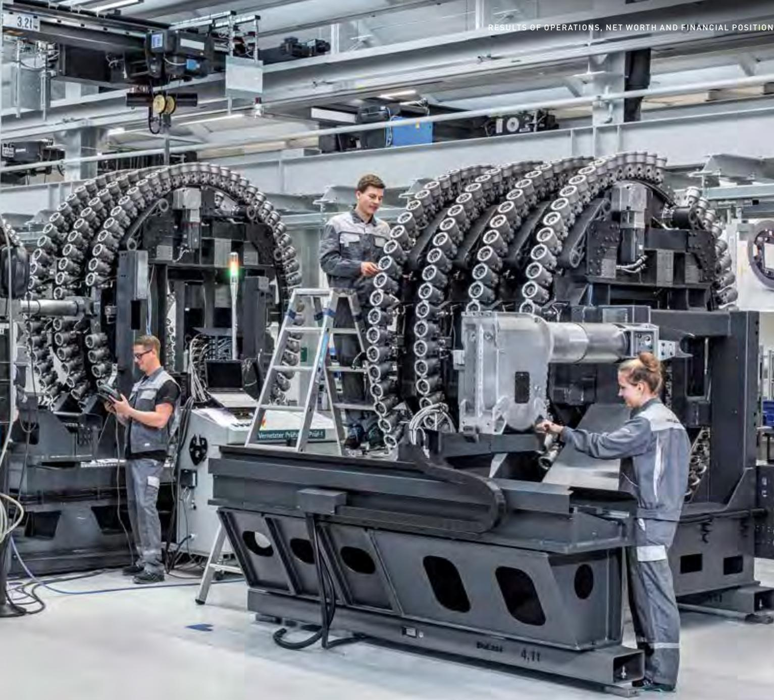
**High-precision work at DMG MORI:** Employees at DECKEL MAHO in Pfronten adjust the modular, patented wheel magazine with space for over 450 tools for the duoBLOCK series. In the pre-assembly, DMG MORI already lays the foundation to ensure that our core components are absolutely precise and extremely robust.
