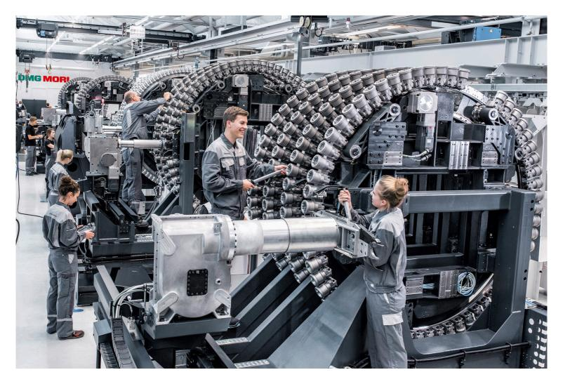
**High-precision work at DMG MORI:** Employees at DECKEL MAHO in Pfronten adjust the modular, patented wheel magazine with space for over 450 tools for the duoBLOCK series.
