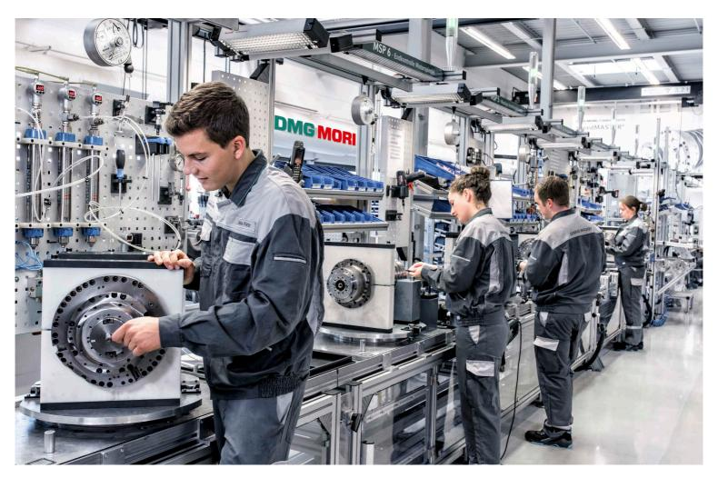
**Cycle-timed spindle assembly:** DMG MORI employees assemble more than 4,000 speedMASTER spindles per year on modern high-tech workstations. As the centerpiece of every machine tool, motor spindles have an enormous impact on the precision and surface quality of the workpieces. Their sturdiness and long-term precision directly impacts the reliability and utilization ratio of machine tools.
