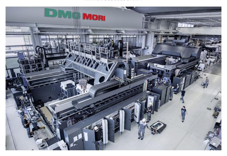
**Machines for processing large-size workpieces:** In the XXL machine assembly hall, DMG MORI produces, among others, the DMU 600 Gantry. The 5-axis universal processing center is comparable to a two-storied single-family house in size.
