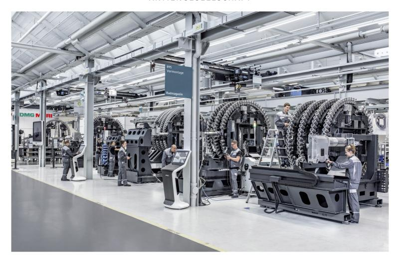
**High-precision work at DMG MORI:** In state-of-the-art and energy efficient assembly halls, employees adjust the modular, patented wheel magazine with space for over 450 tools.
