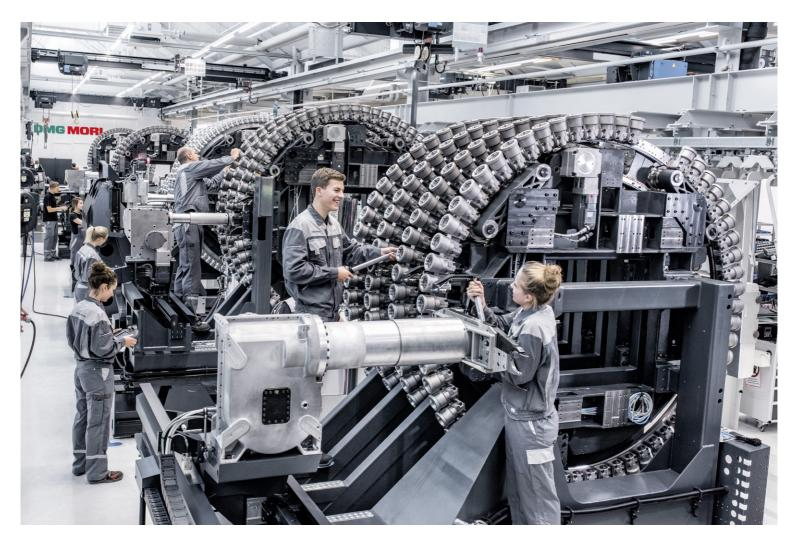
**High-precision work at DMG MORI:** Employees at DECKEL MAHO in Pfronten adjust the modular patented wheel tool magazine for the duoBLOCK series with space for over 450 tools.
