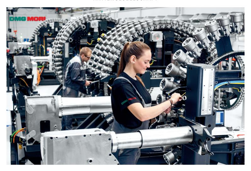
**DMG MORI High-precision work:** Franziska Dreier, industrial mechanic at DECKEL MAHO in Pfronten, adjusts the modular, patented wheel tool magazine for the duoBLOCK series with space for over 450 tools.
