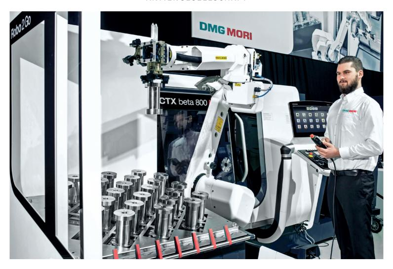
**Focus on automation:** DMG MORI offers automation solutions that are optimally adjusted to each other as the Robo2Go – a robot cell for standard automation of universal turning machines. In the future, every machine of DMG MORI should be equipped with automation.
