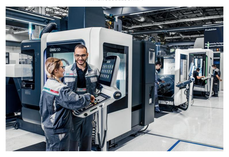
**Attractive Employer:** At DECKEL MAHO in Seebach apprentices are readied early for Indusrie 4.0. Laura Hermann and Dimitri Guloglou programme the DMU 50, a universal milling machine for 5-axis machining, via the innovative APP-based control and operating software CELOS.
