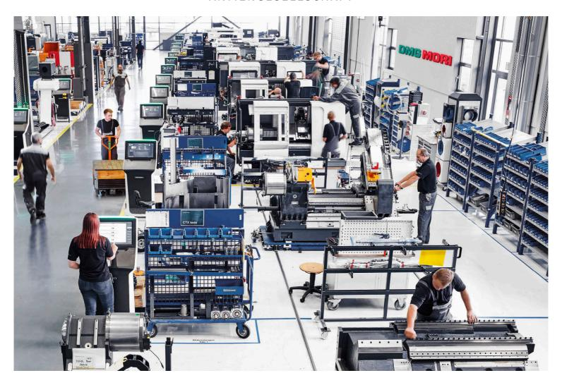
**Efficient line assembly:** In 14 cycles the staff of GILDEMEISTER Drehmaschinen GmbH in Bielefeld manufactures the universal lathe NEF 400 amongst others. Standardized processes guarantee high efficiency and process reliability.
