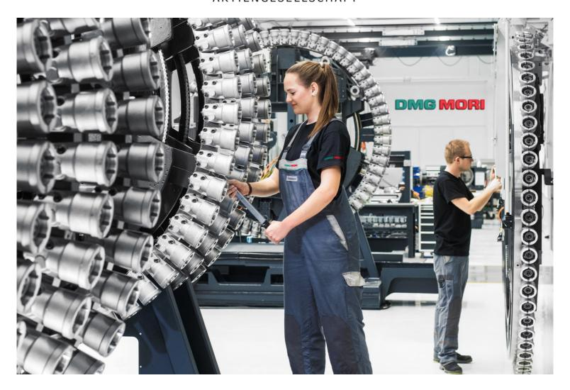
**High-precision work:** Franziska Dreier, industrial mechanic at DECKEL MAHO in Pfronten, adjusts the modular, patented wheel tool magazine for the duoBLOCK series with space for over 450 tools.
