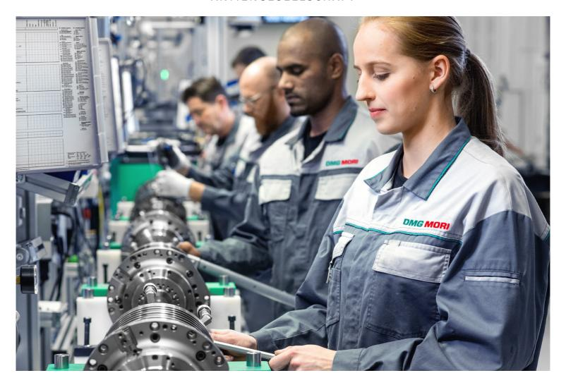
**Cycle-timed spindle assembly:** At modern high-tech workplaces at DECKEL MAHO in Pfronten the aspiring mechatronics technician Sarah Menhofer (front) and her colleagues manufacture the speedMASTER spindle. Already more than 3,000 DMG MORI machines are equipped with speedMASTER spindles.
