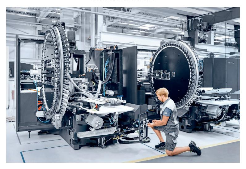
**Dynamic and precise:** A DMG MORI employee adjusts the hydraulic settings of the NHX 4000 horizontal machining centre. The high-tech machine is produced by DECKEL MAHO in Pfronten and is used in the automotive industry amongst others.
