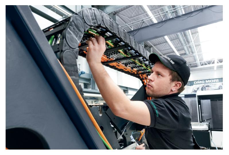
**Quality assurance:** An employee of DECKEL MAHO in Seebach screw connecting the energy supply to the DMF 260 | 11 universal milling machine, which is used in aviation and aerospace among other industries.
