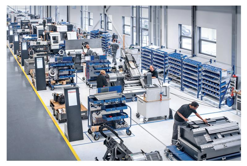
**Efficient flow assembly:** Employees of GILDEMEISTER Drehmaschinen GmbH in Bielefeld assembling the CTX beta 800 TC and other machines in 14 cycles. This high-precision turning and milling centre won the Innovations Prize in 2015 and it is used particularly in mechanical and plant engineering.
