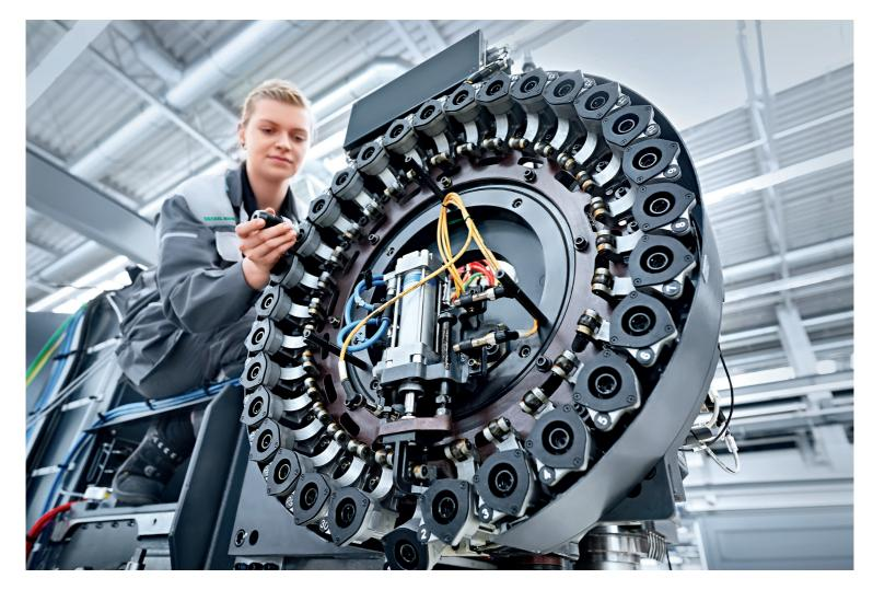
**Precision technology:** An employee of DECKEL MAHO in Seebach aligning the tool changer of an HSC 30 *linear*. This high-speed cutting precision centre is used especially in modern medical technology for the production of joint components or surgical instruments.
