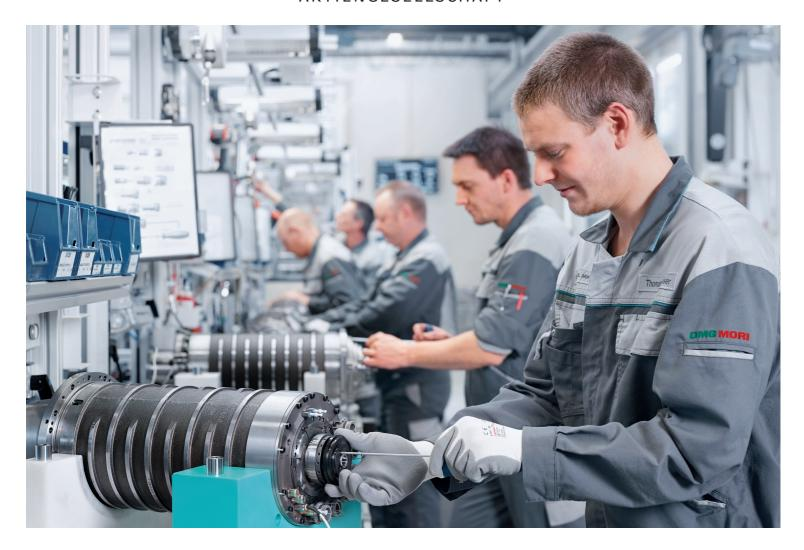
**Cycle-timed flow assembly:** Employees of DECKEL MAHO in Pfronten inspect the settings of motor spindles – the heart of every machine tool.
