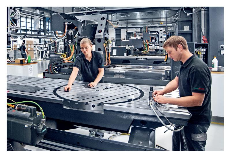
**Basic structure:** Two employees of DECKEL MAHO Seebach install an integrated machining table and a laser tool measurement system on a DMF 260 I 11. This universal milling machine is used in tool building and mould making, among other uses.
