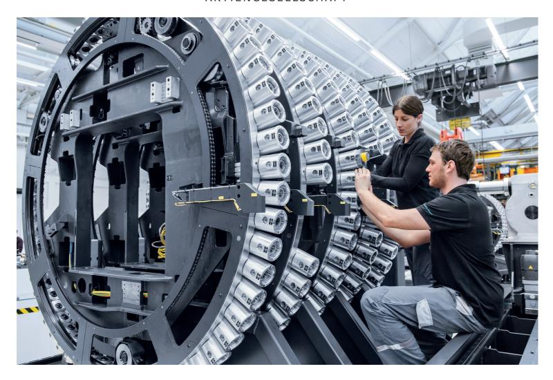
**High-tech from DMG MORI:** Two employees at DECKEL MAHO Pfronten adjust a wheel magazine with space for up to 453 tools for a DMC 80 H *linear* universal milling machine.
