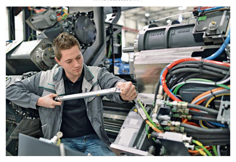
**Precision work:** At the production plant of GILDEMEISTER Drehmaschinen GmbH in Bielefeld, an employee installs compression hoses on the CTX gamma 2000 TC *linear*.
