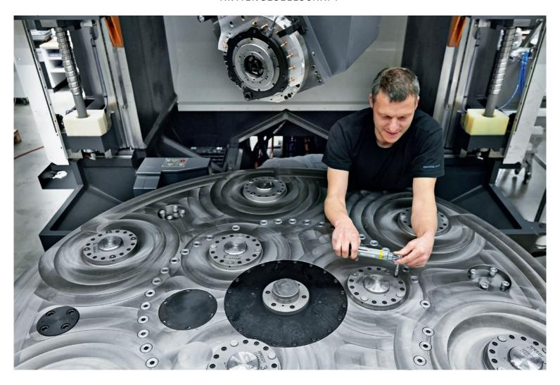
**High-tech machines of DMG MORI:** At the production plant of DECKEL MAHO in Pfronten, an employee adjusts bushes on the 5-axis portal machine DMC 210 FD.
