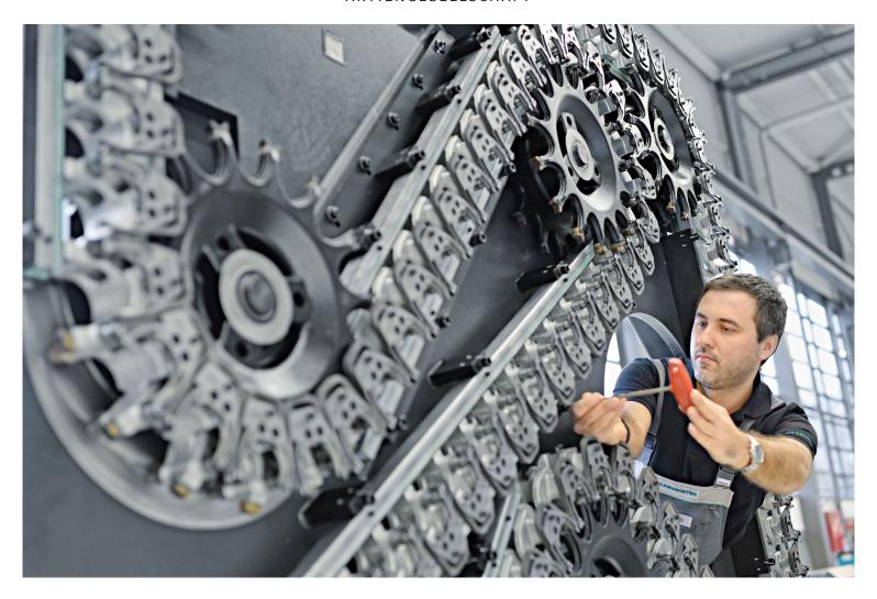
**Pioneering high-tech-machines by DMG MORI:** An employee of the GILDEMEISTER Drehmaschinen in Bielefeld assembles and adjusts of a chain magazine.
