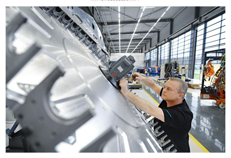
**Adjustment of a tool magazine:** At the Bielefeld production site, pioneering lathes are manufactured e.g. for toolmaking and mould construction, as well as for the automobile industry.
