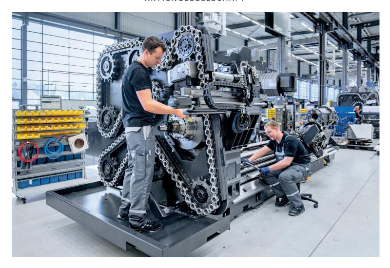
**Complete machining on a single machine:** Two employees at GILDEMEISTER Drehmaschinen GmbH in Bielefeld fit a universal lathe with a chain magazine.
