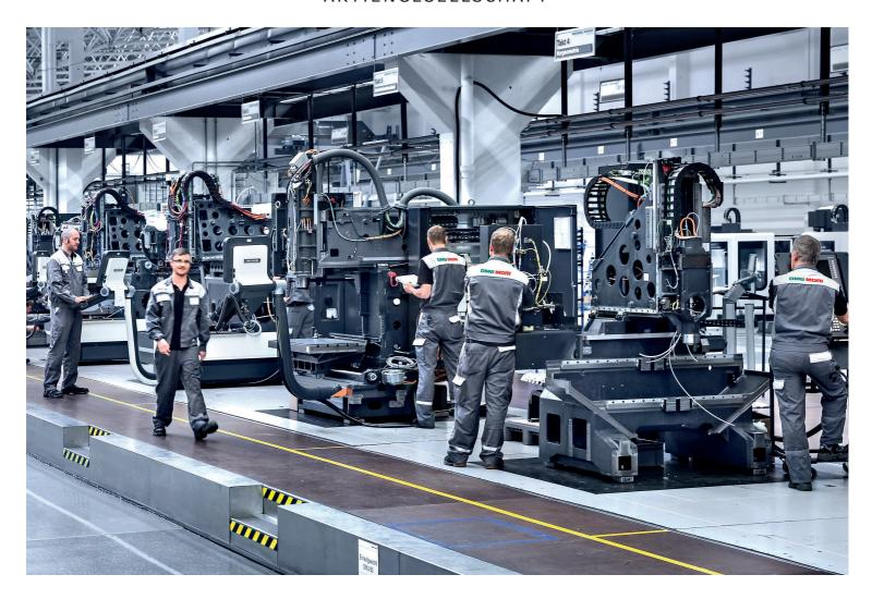
**Complex production processes:** The flow assembly at DECKEL MAHO in Seebach paves the way for the efficient production of high-tech machine tools.
