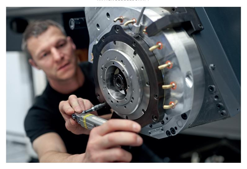
**High-tech machines from DMG MORI:** Assembly of a spindle head for large-scale machines in the production plant at DECKEL MAHO Pfronten GmbH.
