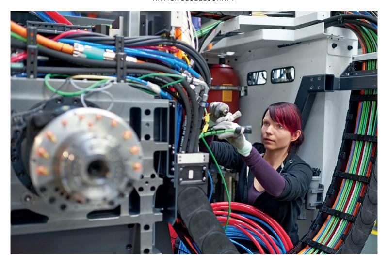
**High-tech machines from DMG MORI for the automotive industry:** Cable assembly on a DMC 60 H linear *linear* in the production plant at DECKEL MAHO Pfronten GmbH.
