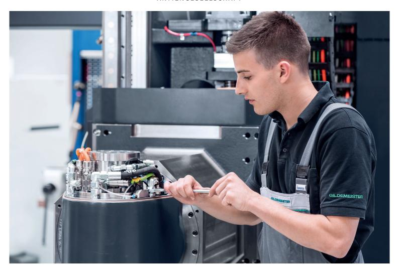
**Precision work:** A GILDEMEISTER Drehmaschinen GmbH employee in Bielefeld fits hydraulic hoses to the spindle on a tool carriage. This is fitted to the CTX gamma 2000 universal lathe, for example, on which hydraulic components for the automobile industry are fabricated.
