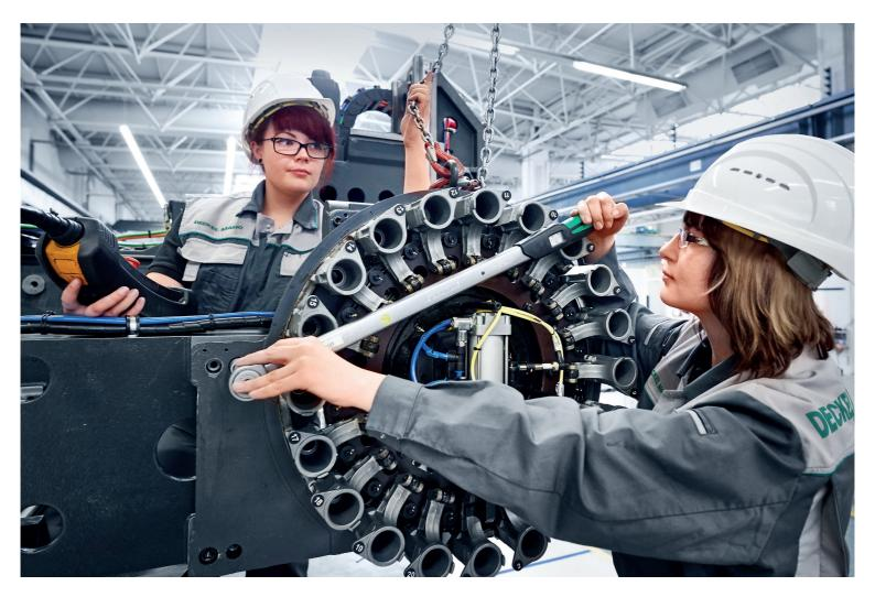
**Teamwork:** Two apprentices at DECKEL MAHO Seebach install the tool changer on a DMC 1150 together. This universal milling machine is mostly used in toolmaking and mouldmaking.
