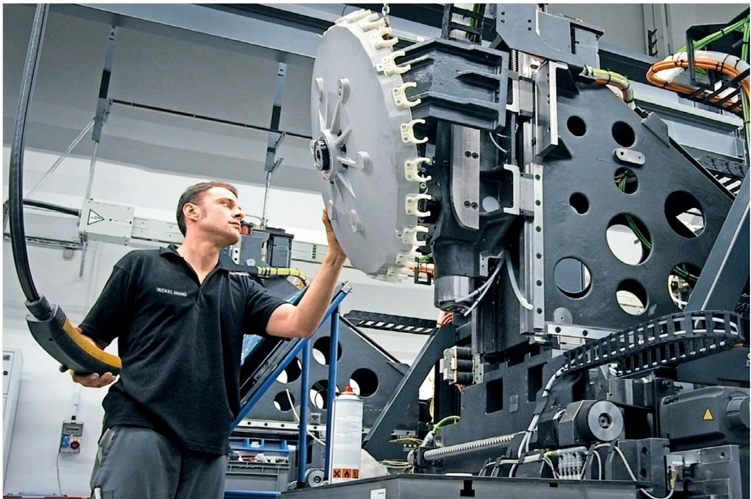
**Assembly of a tool changer:** Dirk Ziegler, assembly fitter at DECKEL MAHO Seebach GmbH, installs a tool changer on a MILLTAP 700.
