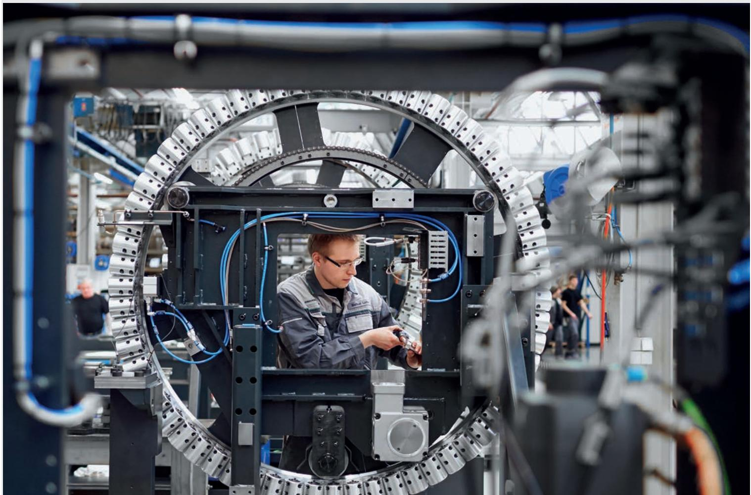
**Big dimensions:** Markus Lotter, industrial mechanic at DECKEL MAHO Pfronten GmbH, assembles a tool magazine for a DMC 60 H *linear*.
