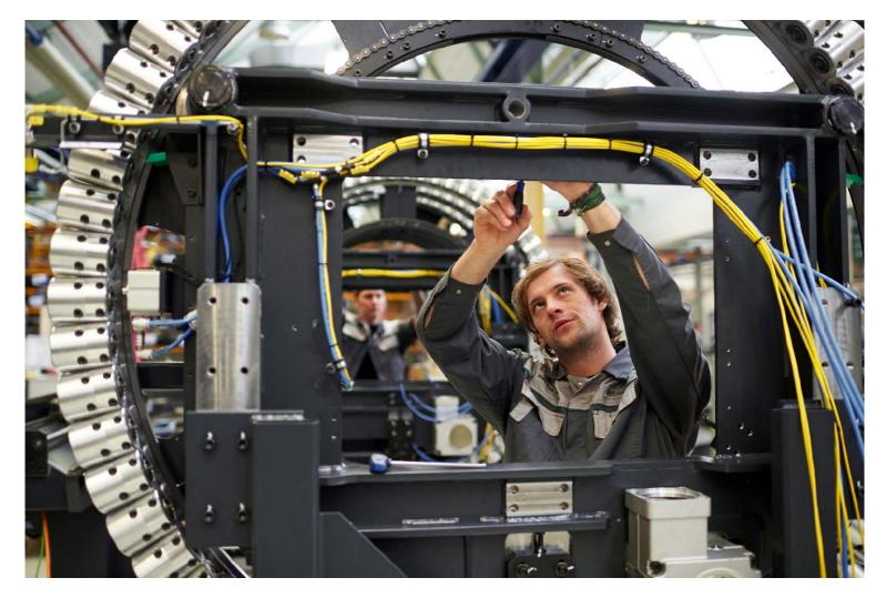
**Technology and innovation by DMG MORI:** An industrial mechanic installs a tool magazine on a DMC 60 H *linear* in the production plant for large machines in Pfronten.
