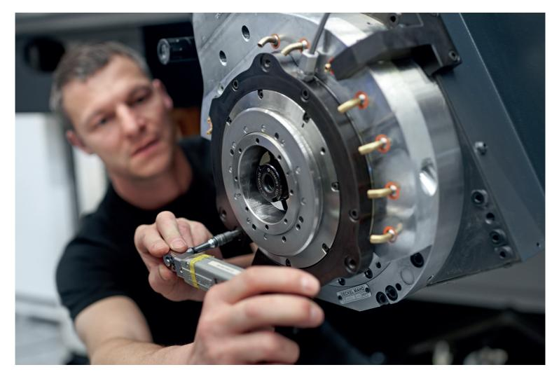
**High-tech machines by DMG MORI:** Installation of a headstock for large machines in the DECKEL MAHO Pfronten GmbH production plant.
