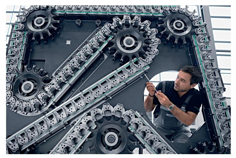
**High-tech machines by DMG MORI:** Installation and adjustment of a chain magazine at GILDEMEISTER Drehmaschine GmbH in Bielefeld.
