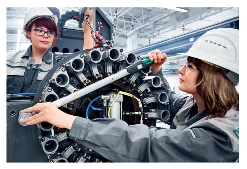
**Precision work:** Two employees of DECKEL MAHO in Seebach assemble the tool changer of a DMC 1150 V. This vertical machining centre is used especially in tool and mould making.
