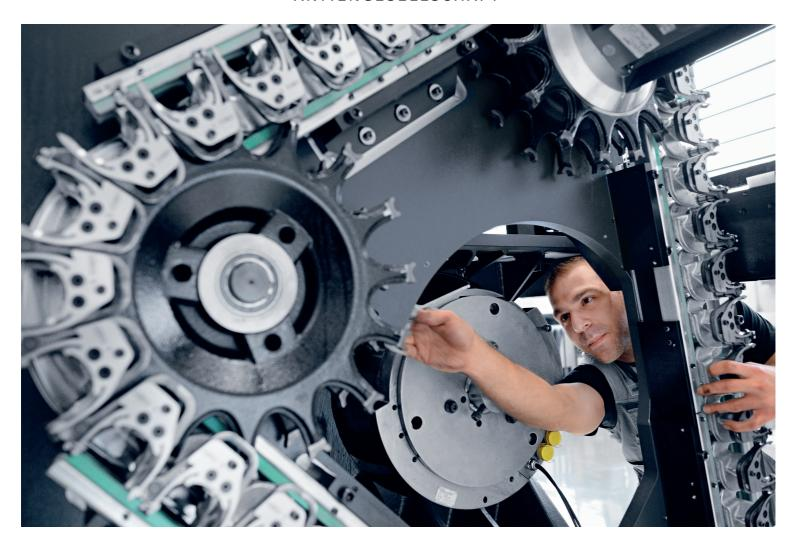
**High-tech machines of DMG MORI:** An employee of GILDEMEISTER Drehmaschinen GmbH in Bielefeld adjusts a tool magazine for the CTX gamma TC of the 2nd generation. The pioneering turning / milling machine is manufactured, for example, for the complete machining of components in the automotive industry.
