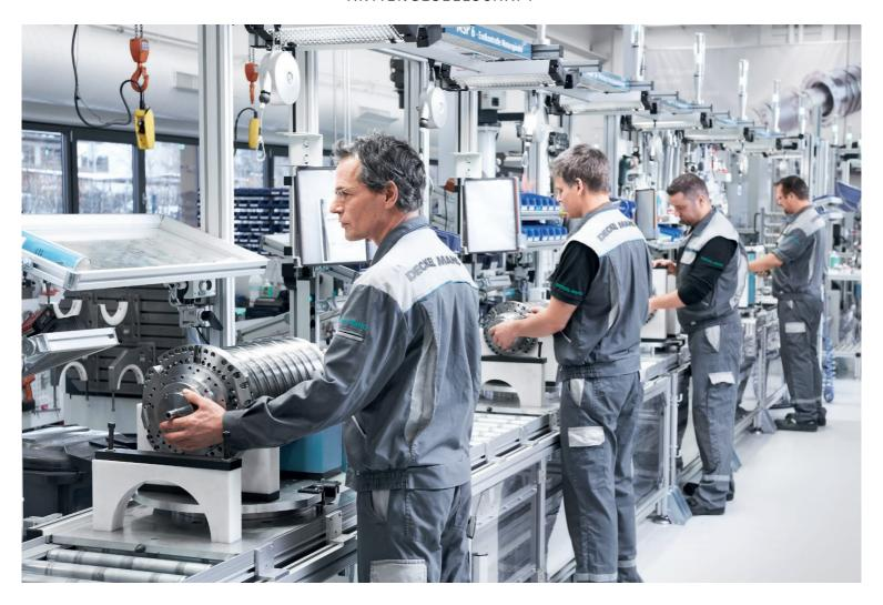
**Cycle-timed flow assembly:** employees of DECKEL MAHO in Pfronten checking the settings of a motor spindle – the heart of any machine tool.
