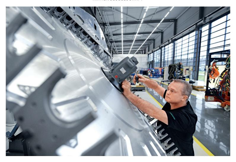
**Adjustment of a tool magazine:** at the production site in Bielefeld, pioneering turning machines are manufactured, e.g. for tool building and mould making as well as for the automotive industry.
