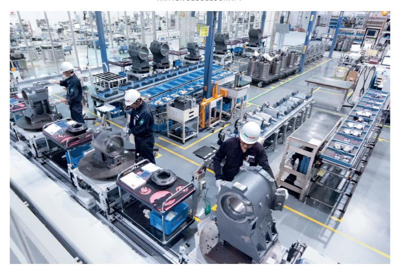
**Precision assembly:** at the Japanese plant of DMG MORI SEIKI COMPANY LIMITED in Iga, the main spindles for turning machines of the NLX series are assembled, which are used especially in the automotive industry.
